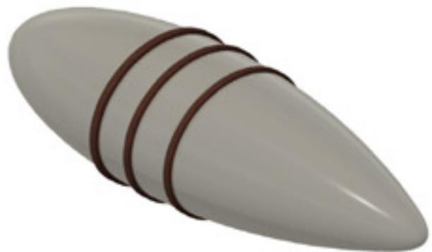
Fig.16 Projected View of the Ring Structured Aerostat requiring the winch to be mounted on top of the tower. This arrangement eliminates the risk of the winch becoming fouled with the power carrying cables attached to the tower.
